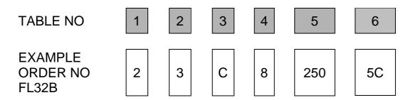
**Example Order No. =** Type FL32B; two floats; three contacts; 1 1/2" B.S.P process connection ; ST.ST.316 material ; 250mm long ; 5 meter PVC cable connection.
